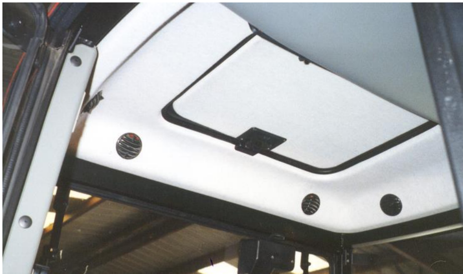
Rear recirculation louvers in place.
