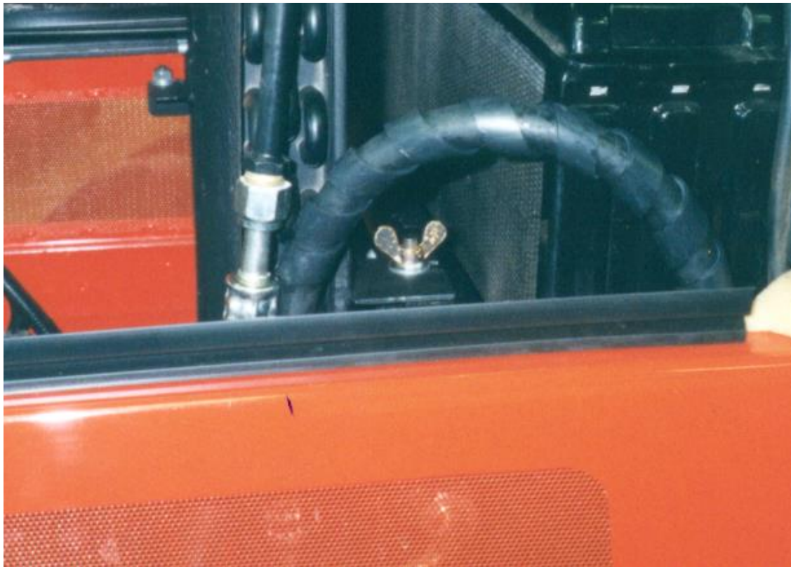
Left side of condenser showing wing nut on radiator frame securing rear condenser bracket.
